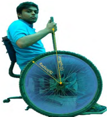
Fig. 1 Changing hand position on the levers varies mechanical advantage of the drive train
