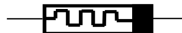
Fig.1 We use the following convention when possible: when a positive voltage is applied to the second (plain without lining) terminal with respect to the terminal denoted by the black thick line, the memory device goes into a state of high resistance.
