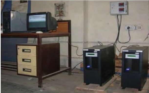
Fig. 3. Setup of Solar & Wind PCUs with Grid & PC for data Logging
