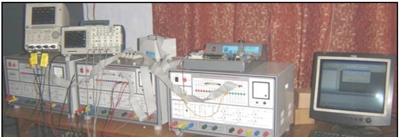
Fig. 8 The quasi-six phase voltage source inverter set-up
