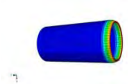
Fig. 3(d) Stresses in steel cylinder
